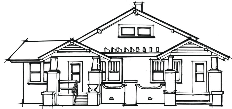
Figure 6: This Craftsman duplex at 415-417 N. Walnut features shallow gabled roofs, exposed rafter tails and square brick piers.
