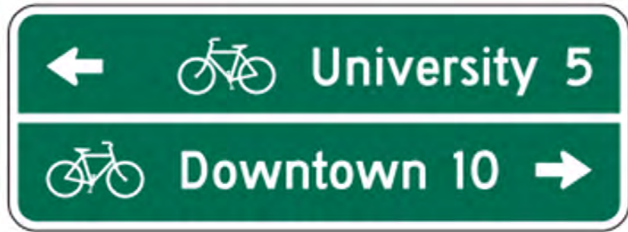
Typical guide sign (D1-2C) for bicycle facilities (MUTCD, 2009)
