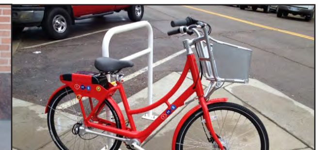
Figure 3.7 - “Inverted U” Bicycle Rack (Excellent Design)
